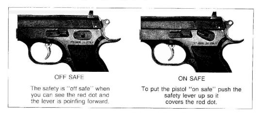
The safety can be operated with the hammer cocked or not cocked and with the pistol loaded or unloaded. There is not a magazine safety, so the pistol may be fred with the magazine removed.
